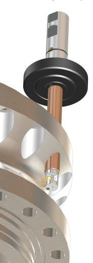
**Steiner Solution:** A fully automatic and mechanically activated Flywheel Autofacer® from Steiner Technologies utilizes the machine's spindle inertia to open & close the cutting blade. The CNC machine used was a Doosan 4020 vertical mill running at 250 SFPM with a feed rate of .0031 IPR.
